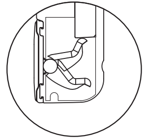
Pressure lever in the housing (Pressure lever in normal position without load!)
